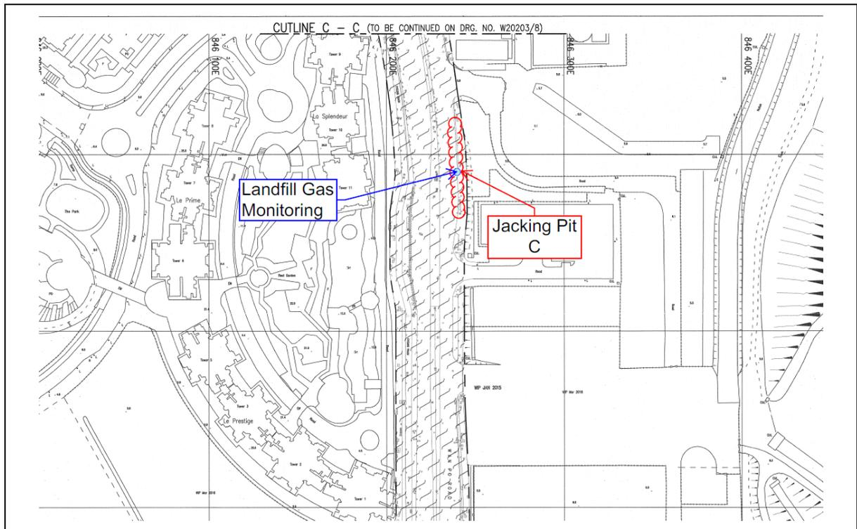
Figure 4.5 Monitoring Location – CH.A 19+15 ~19+50 (Pit C)
