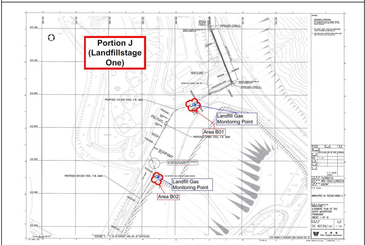
Figure 4.10a Monitoring Location – Landfill Stage 1 (Area B01-B02)
