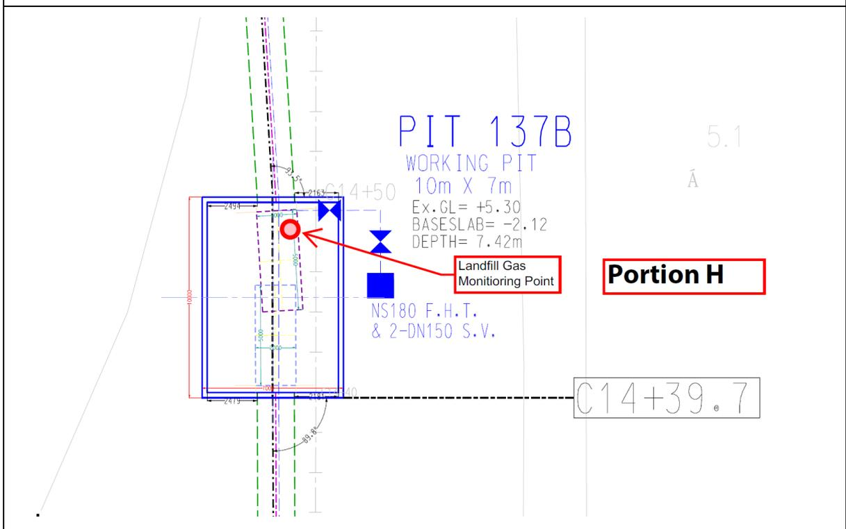
Figure 4.8b Monitoring Location – Pit 137B (137 Pit B)
